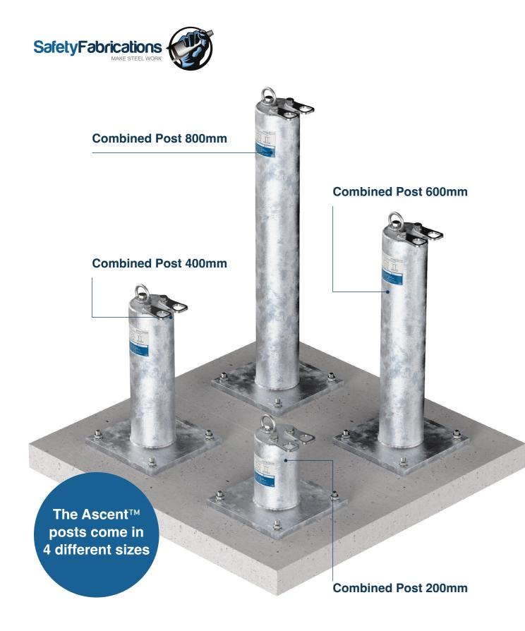
Ascent Fall Protection Posts are manufactured from Galvanised Mild Steel. The Posts are tested as a complete anchor system to reinforced concrete, but are typically supplied as a seperate Anchor Device & Anchor Point (S) with the specialist installer providing the permanent fixing element suitable to the background to which the anchor device is to be affixed. All Ascent™ products have been approved through the necessary safety & structural calculation.
